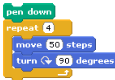
Fig. 3. Lesson-4, showing a repeat-block for iteration
